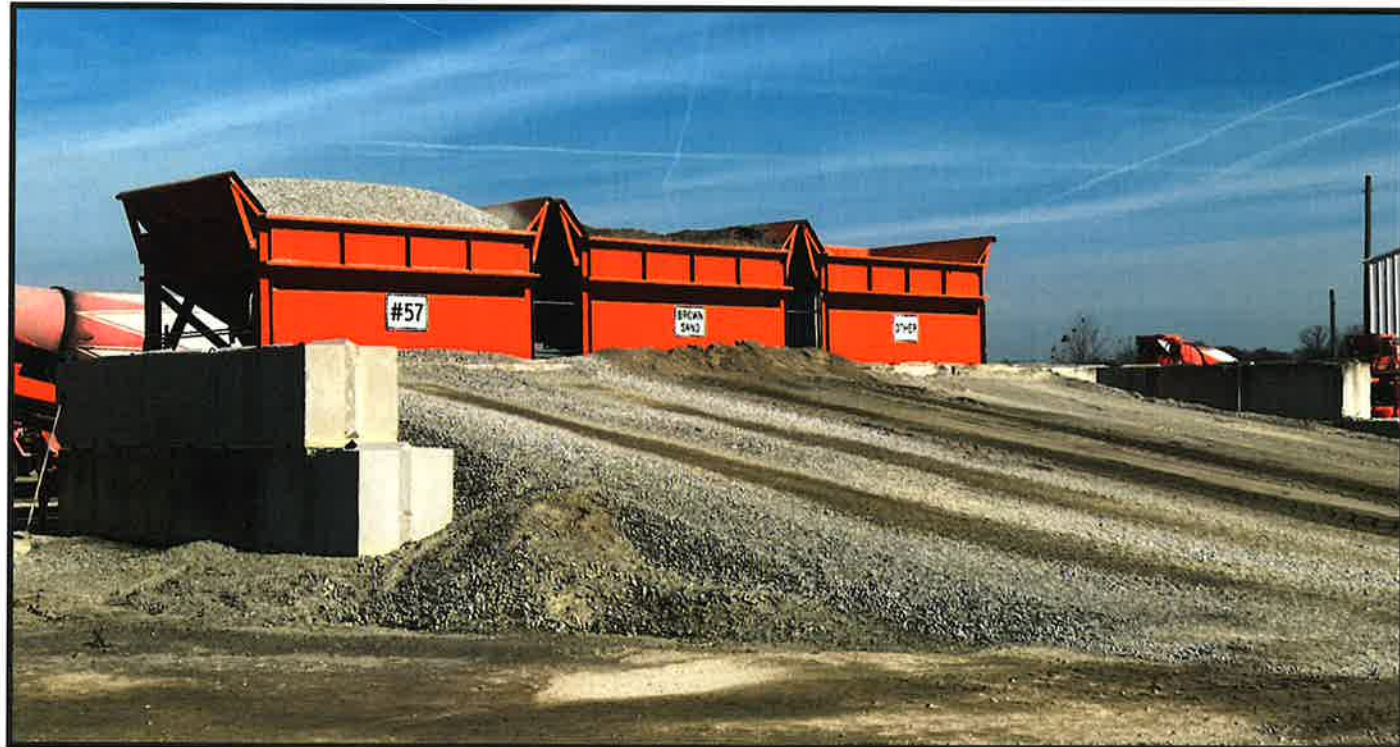
Picture 5: Example Ground Storage Bins and Ramp
