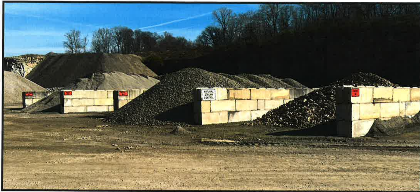
Picture 4: Example Retail Aggregate Sales Bunkers
