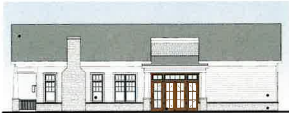
VINYL WINDOW FIBERGLASS DOOR 4 SIDE ELEVATION 3/32" = 1'-0"
